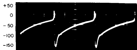
FIG. 8-A GRID (PIN #1) V-1 BLOCKING OSCILLATOR P.R.F. = 50kc
