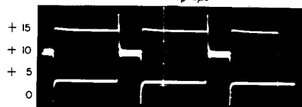
FIG. 8-E GRID (PIN #1) V-3 WITH CATHODE (PIN #7) SUPERIMPOSED MULTIVIBRATOR P.R.F. = 50kc T_p = 5\mu s
